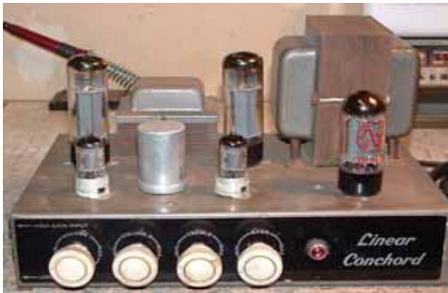
Liner Concord 30 Amplifier
