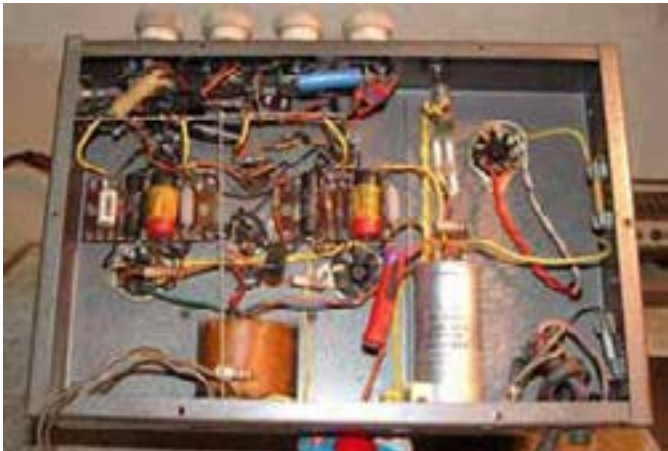
Hand Wired Main Chassis
