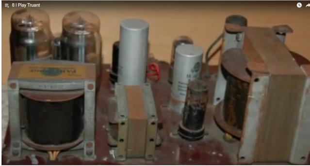
**Amplifier Using PX4 Valves**
