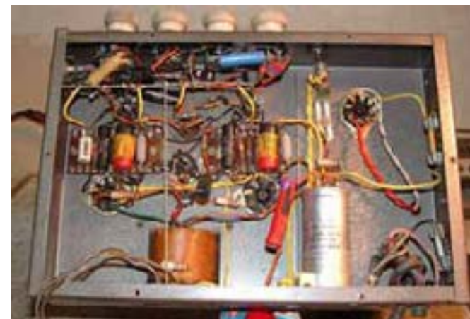
Hand Wired Main Chassis
