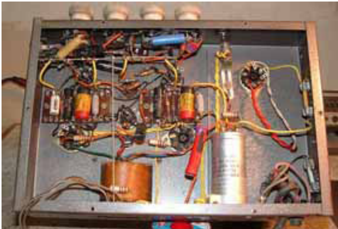
Hand Wired Main Chassis
