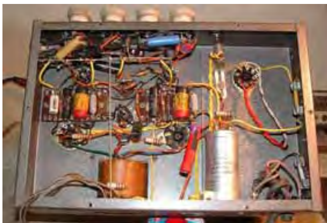
Hand Wired Main Chassis
