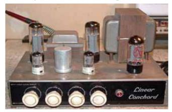
**Liner Concord 30 Amplifier** Top View using EL34 Output valves in push pull
